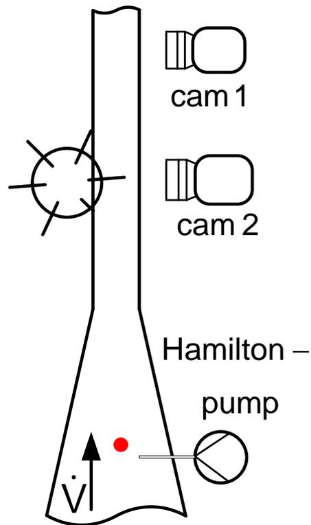
Fig. 1. Sketch of the single drop breakage cell.
