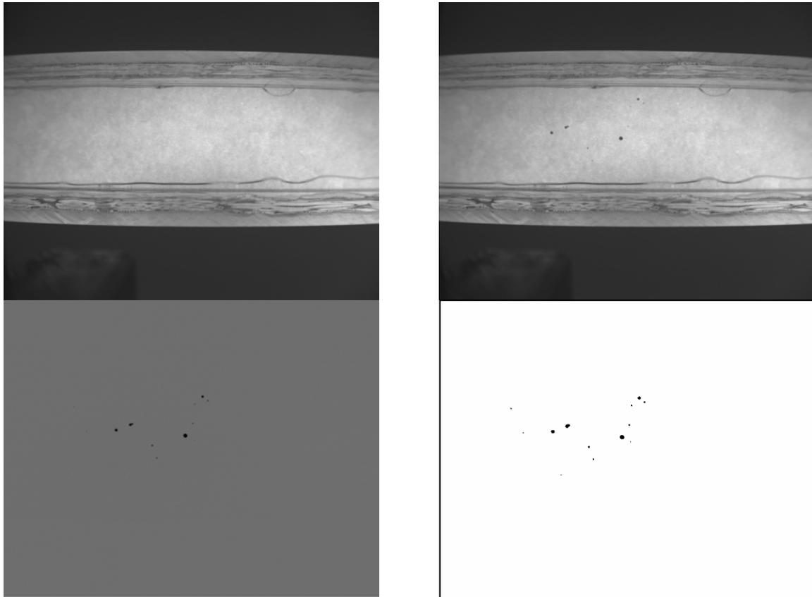
Fig. 2. Pictures of drops in the breakage channel. The picture with drops is subtracted from a reference one without drops. The final picture shows black drops only.
