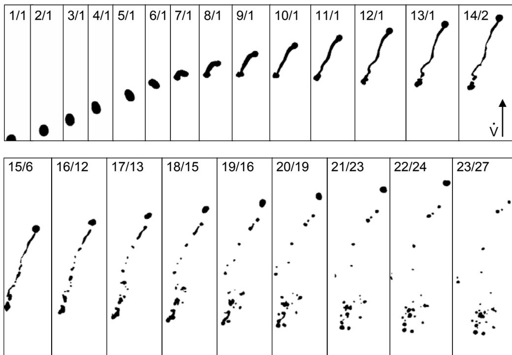
**Figure 2 – Example initial binary breakage with following break-up cascade of 2 mm toluene drop, always with the image number/ number of particles on the image**
