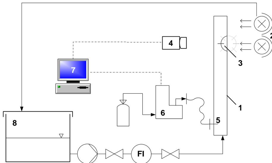
**Figure 1 – Experimental set-up for single drop experiments: (1) breakage cell, (2) illumination, (3) section of a Rushton turbine, (4) highspeed camera; (5) nozzle for drop formation, (6) precision dosing pump, (7) computer control, (8) water storage tank**
