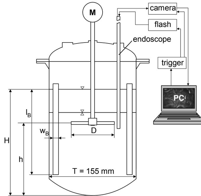
Figure 3 – Experimental set-up and dimensions of the used stirred tank
