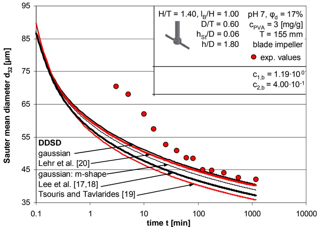
**Figure 9 – Comparison of experimental determined transient Sauter mean diameter and PBE simulations using several DDSs**
