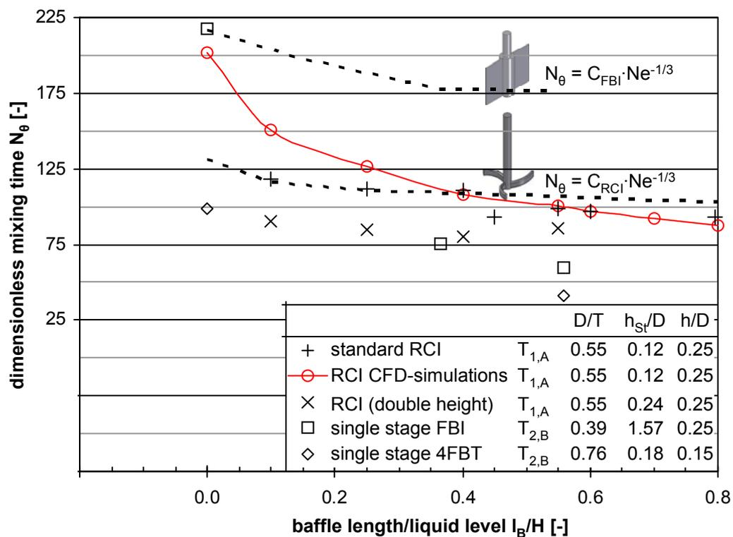
**Figure 6 - Dimensionless mixing time as a function of the baffle length for various single stage impellers in a single phase system at H/T = 2.3**
