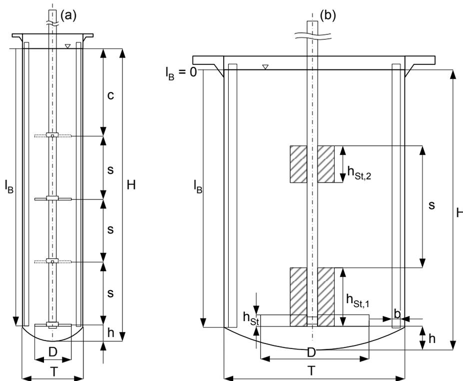
**Figure 1 - Experimental set-up and dimensions of the tanks (configuration A – (a); configuration B – (b)) and the stirrers used**
