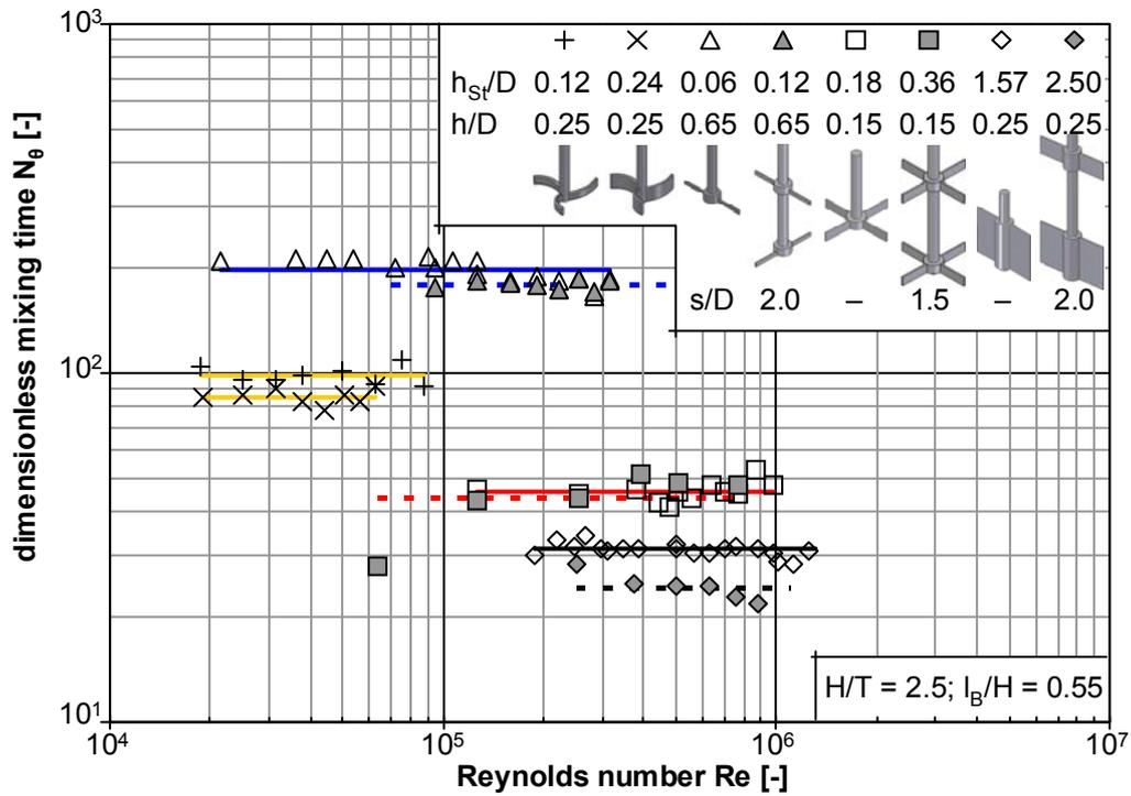
Figure 8 - Dimensionless mixing time over Reynolds number for different stirrer applications in slim reactors
