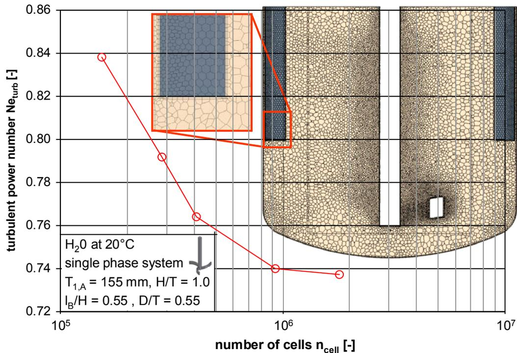
Figure 3 - Sensitivity analysis of predicted power numbers on number of cells used in the grid
