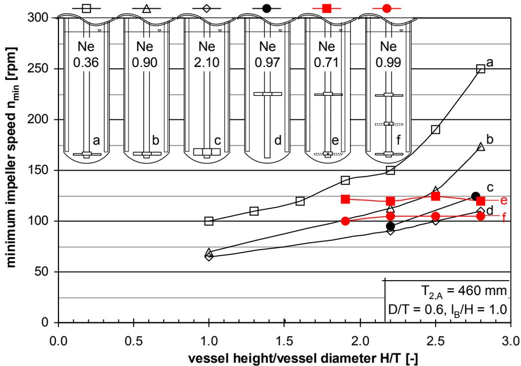
**Figure 13 - Minimum dispersion speed for various single and multi stage crossed blade impeller configurations**
