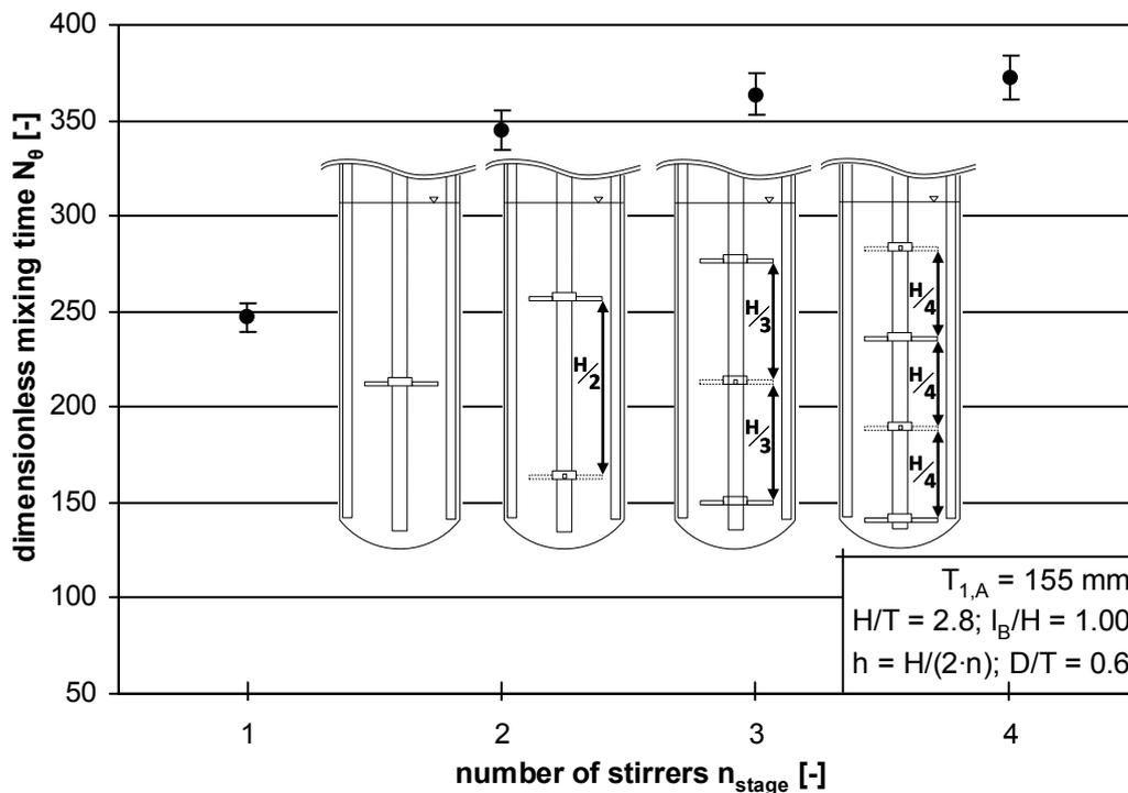
Figure 9 - Dimensionless mixing time for different number of stages with equal stirrer interspaces over the reactor height
