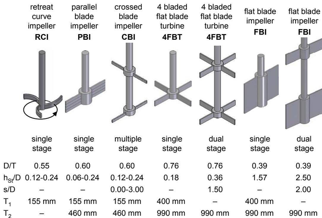
Figure 2 - Design of the radial impellers used
