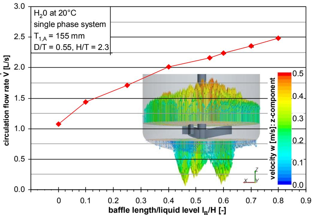
**Figure 5 - Simulations of the axial volume stream as a function of the baffle length for the retreat curve impeller**
