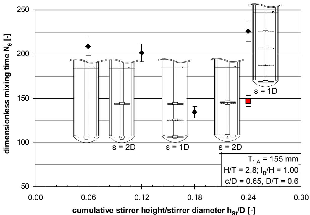
Figure 11 - Dimensionless mixing time for different number of stages
