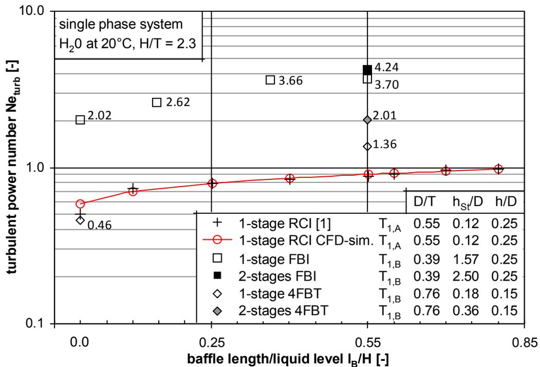
Figure 4 – Comparison of turbulent power numbers for different impellers from experiments and simulations
