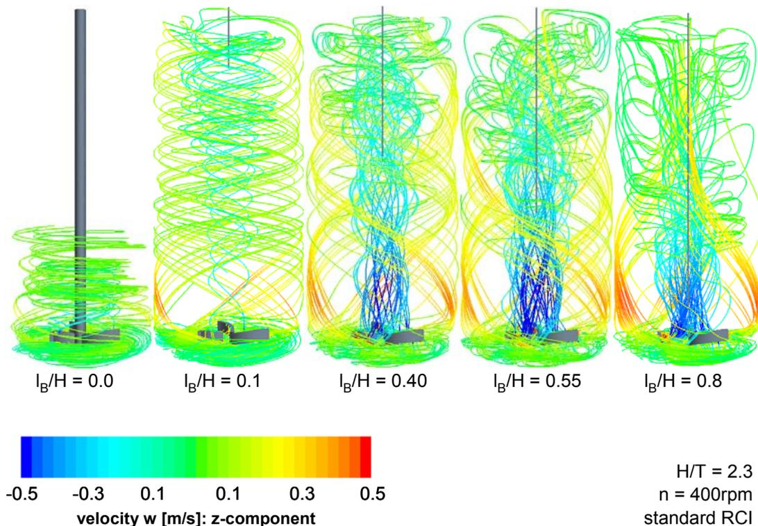
Figure 7 - Streamlines for unbaffled and baffled system with increasing baffle length  $l_B/H = 0.1$  until 0.8
