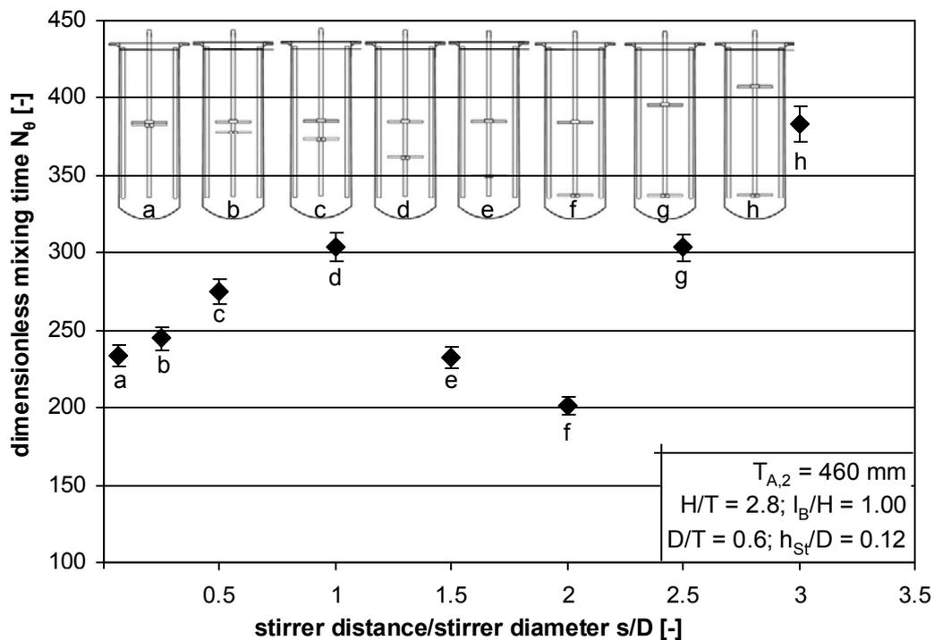
Figure 12 - Influence of stirrer distance of dual crossed blade impellers on dimensionless mixing time
