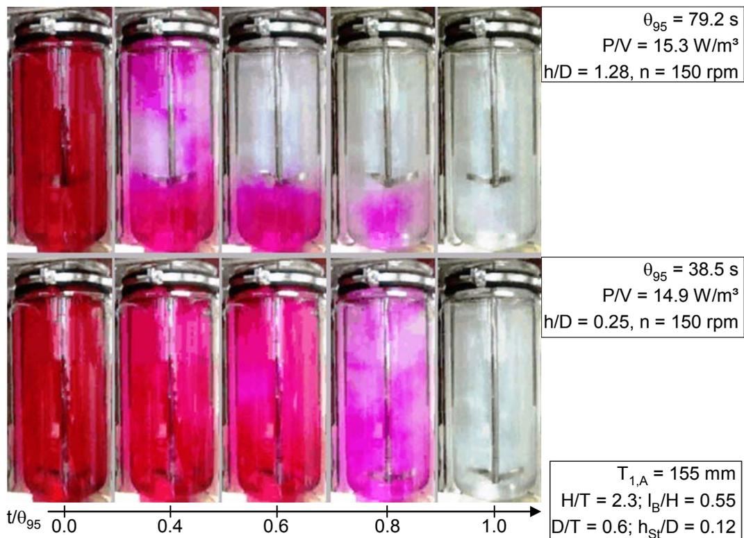
**Figure 10 - Experimental decolorization of retreat curve impeller systems in dependency on stirrer bottom clearance and corresponding fluid flow compartmentalization**
