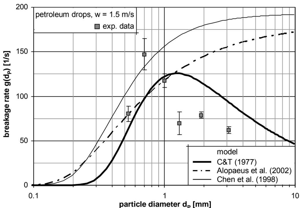
Figure 16 – Comparison of different breakage rates with experimental petroleum single drop experiments, the used parameters in the models are all given in Table 8 in Appendix A (as this study)
