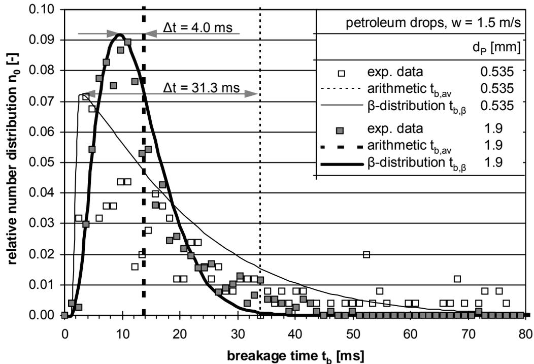
**Figure 9 – Relative number distribution of the breakage time (symbols) and its approximation with a  $\beta$ -distribution (lines) for two different petroleum mother drops at a constant flow velocity.**
