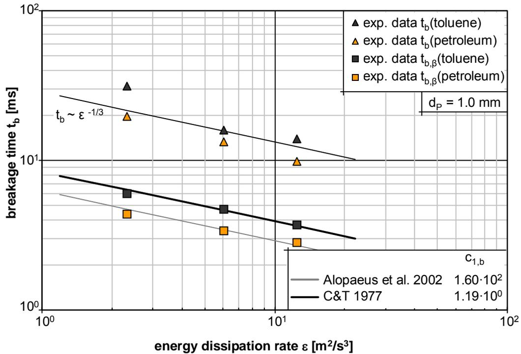
Figure 13 – Dependency of the breakage time on the energy dissipation rate, experimental and model results
