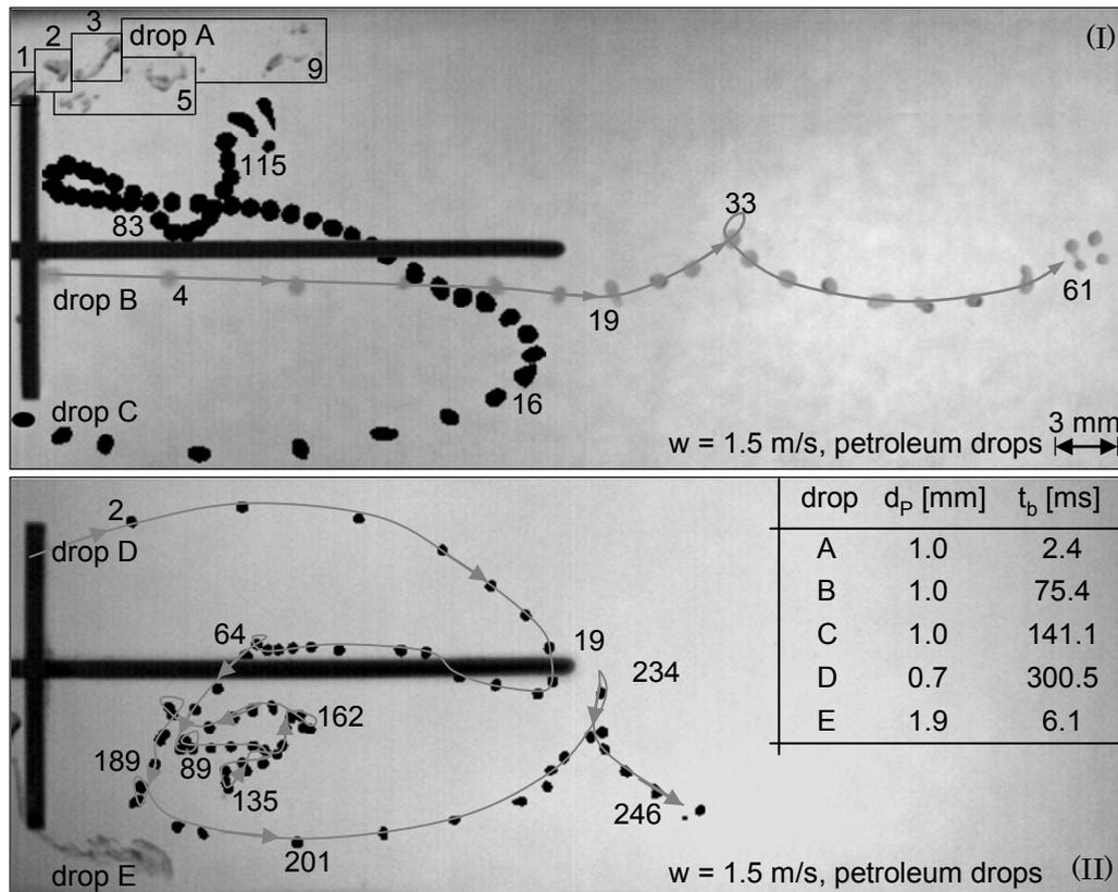
**Figure 10 – Example high-speed images (original – drop A,B,E and after image processing – drop C,D) to illustrate the differences in the breakage time for a constant stirrer speed and a varying mother drop diameter.**
