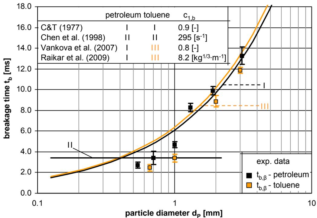
**Figure 12 – Comparison of four breakage time models at a constant superficial velocity of 1.5 m/s (lines) with experimental single toluene and petroleum drops (symbols).**
