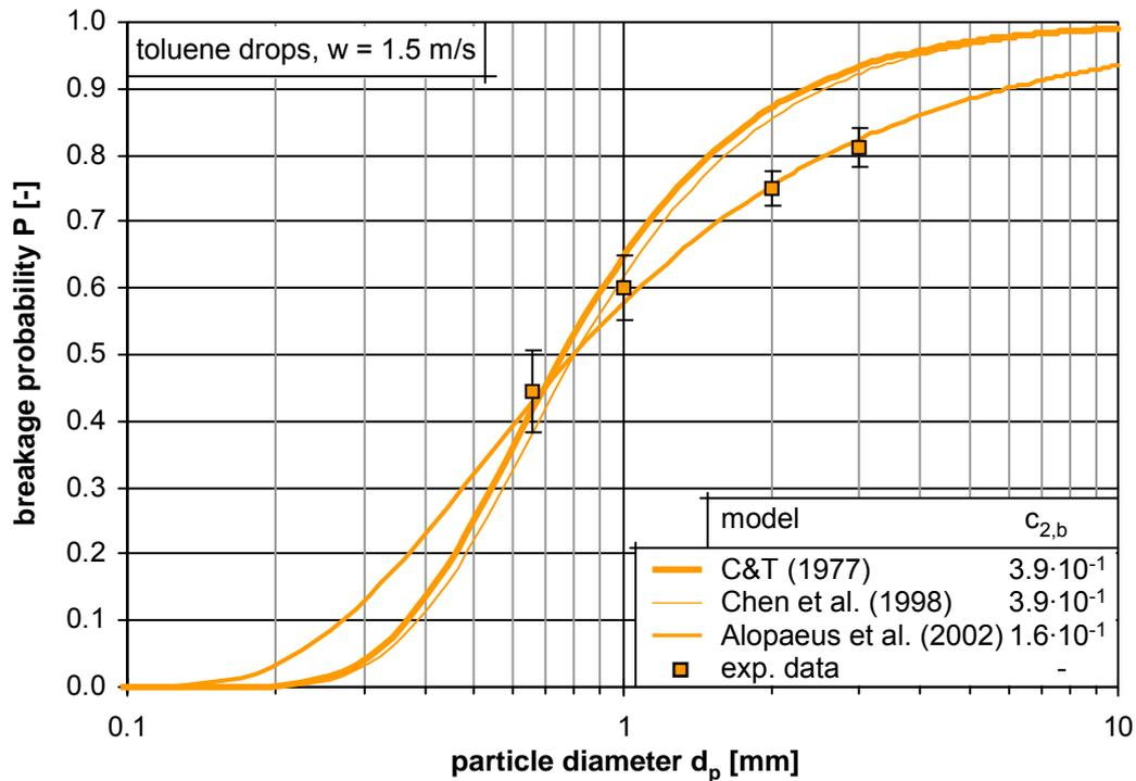
Figure 7 – Comparison of three breakage probability models (lines) with experimental single drop results for toluene drops (symbols).
