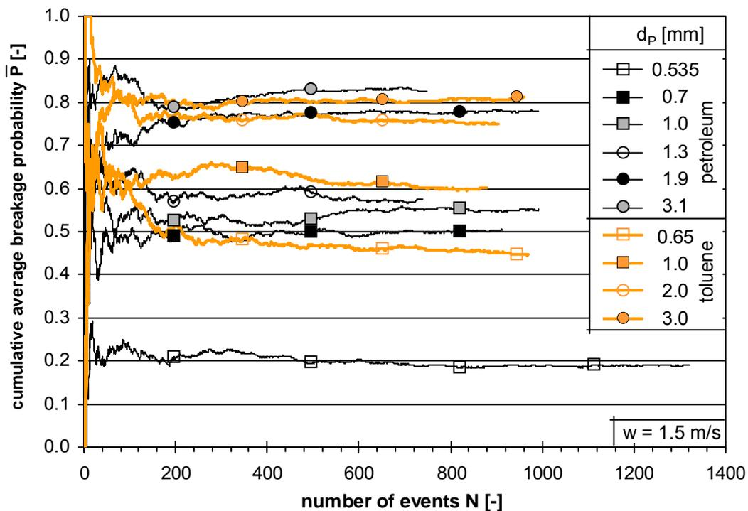
**Figure 5 – Cumulative arithmetic average breakage probability as a function of breakage events of toluene and petroleum drops at a constant flow velocity for different mother drop diameters.**
