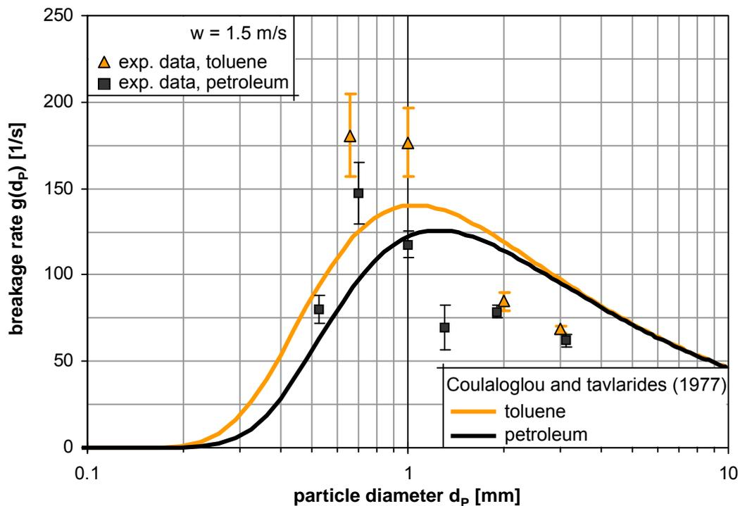
Figure 17 – Comparison of different breakage rates with experimental toluene and petroleum single drop experiments, the used parameters in the models are all given in Table 8 in Appendix A (as this study)
