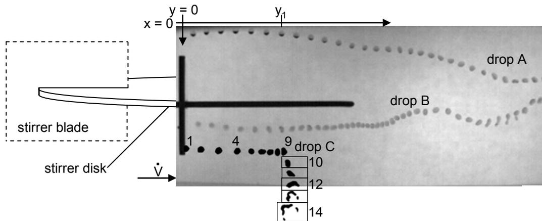
**Figure 3 – Three exemplary toluene drops (drop A and B – original images, drop C – after image processing),  $d_p = 1\text{ mm}$ ,  $w = 1.5\text{ m/s}$ , demonstrating the definition of breakage time and breakage probability.**
