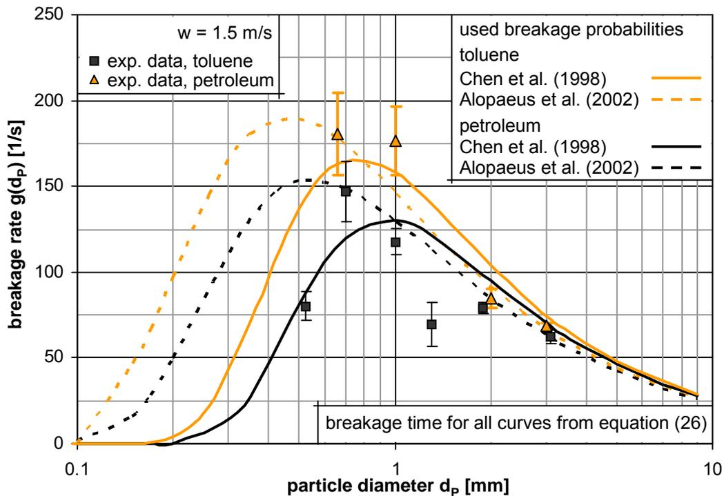
**Figure 18 – A comparison of model data (lines) and experimental results (symbols) is shown. The model consists of breakage probability functions from the literature and the new model approach of the breakage time.**
