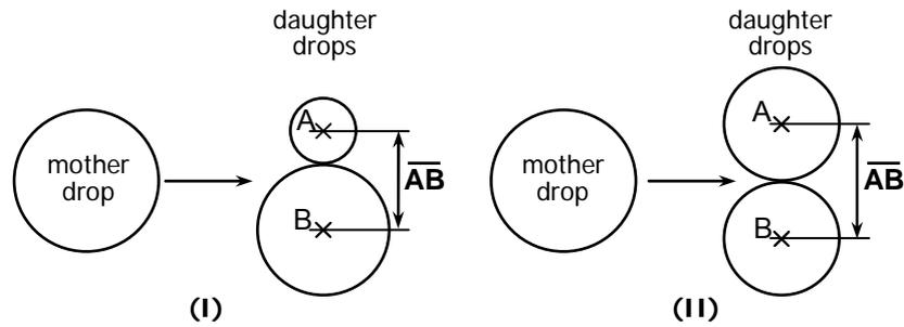
**Figure 1 – Initial distance between the centre points A and B for binary drop breakage: exemplarily unequally sized breakage (I) and equally sized breakage (II). The mass balance is fulfilled for both events.**
