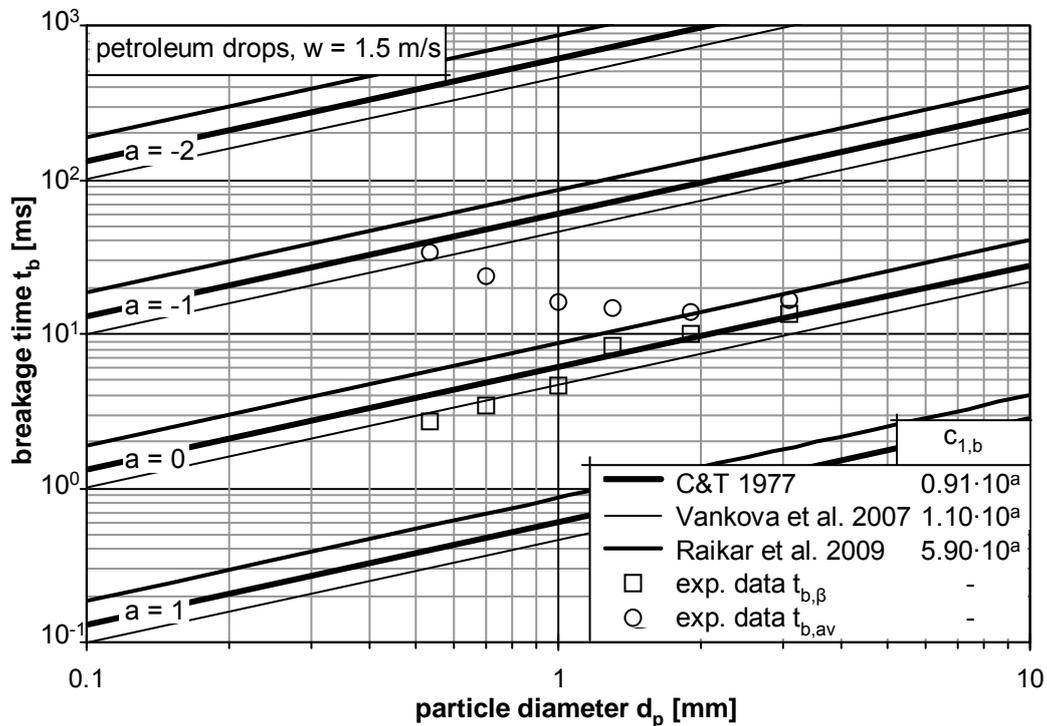
Figure 11 – Comparison of three breakage time models at different parameter magnitudes (lines) with experimental single petroleum drop results (symbols).
