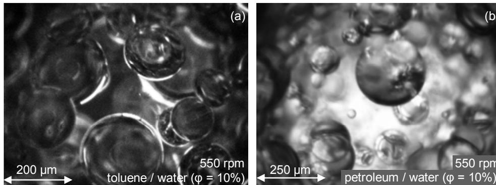
**Figure 4 – Example photos of the analyzed systems in a stirred vessel with a Rushton turbine at a stirrer tip velocity of 1.45 m/s.**
