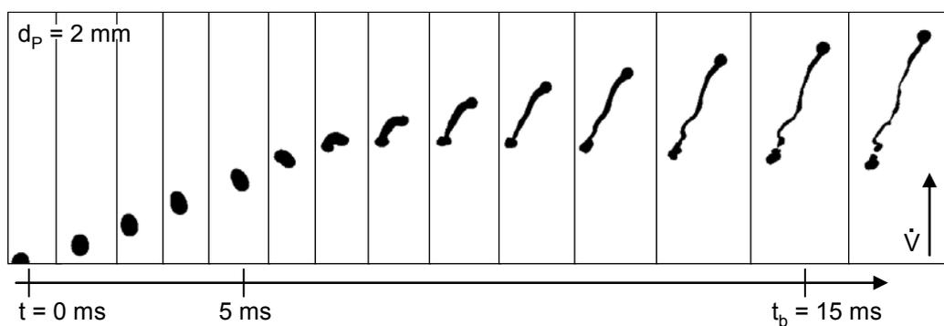
Figure 14 – Example of a breakage event based on drop elongation in the turbulent flow
