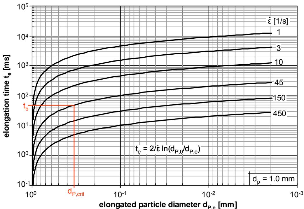
**Figure 15 – Development of the elongation time over the thinning fluid particle thread as a function of the elongation rate  $\dot{\epsilon}$**
