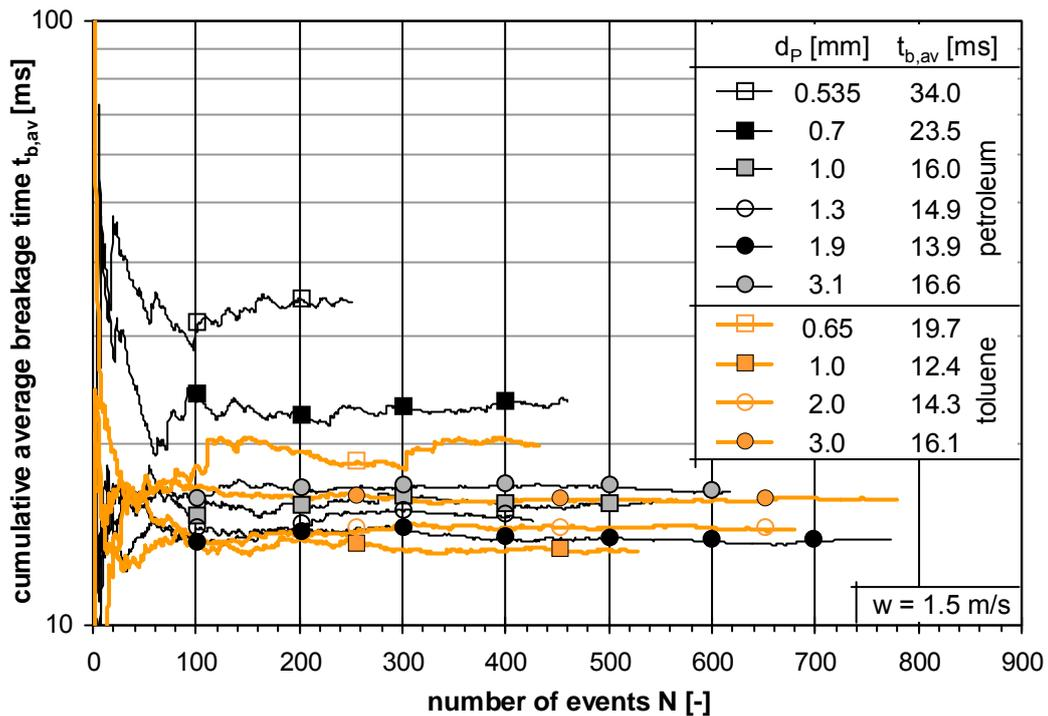
**Figure 8 – Cumulative arithmetic average breakage times as a function of analyzed breakage events for a constant flow velocity and various mother drop diameters.**
