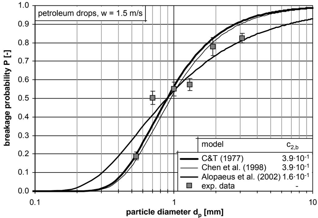
**Figure 6 – Comparison of three breakage probability models (lines) with experimental single drop results for petroleum drops (symbols).**
