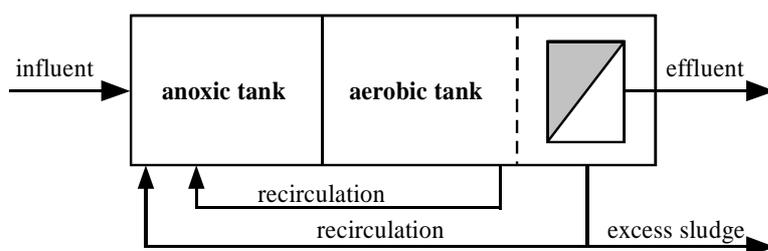
Figure 2: Flow sheet for MBR with basic pre-denitrification (modified Ludzack-Ettinger process).
