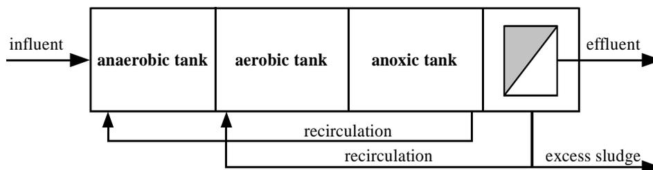
Figure 4: Flow sheet for MBR with enhanced biological phosphorus removal and post-denitrification
