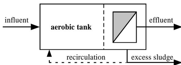
Fig. 1: Basic carbon and nitrogen removal MBR plant scheme
