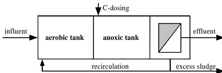
Figure 3: Basic flow sheet for post-denitrification
