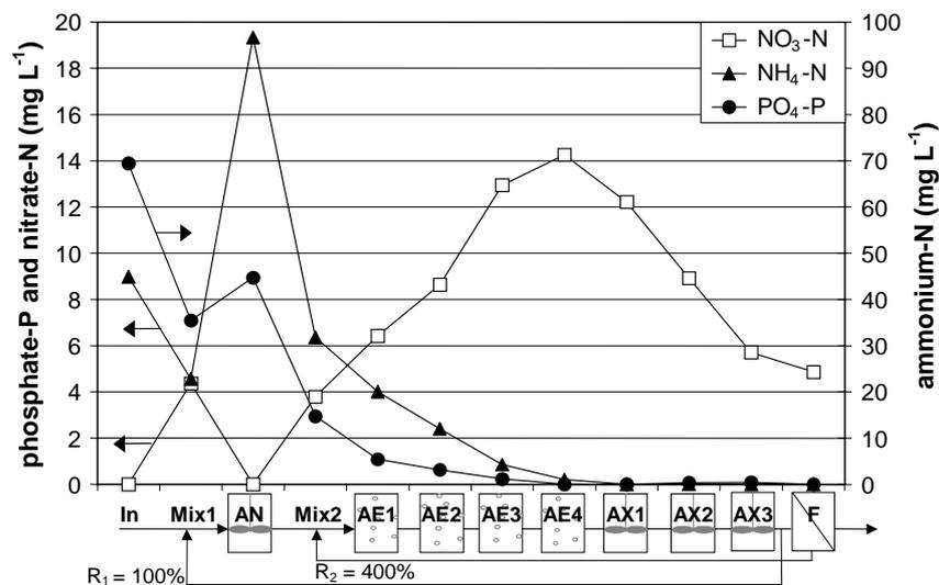
Figure 5: Concentration profiles of phosphate, nitrate and ammonium in a cascaded lab scale MBR operated with municipal wastewater (AN: anaerobic, AE: aerobic, AX: anoxic, F: filter chamber).
