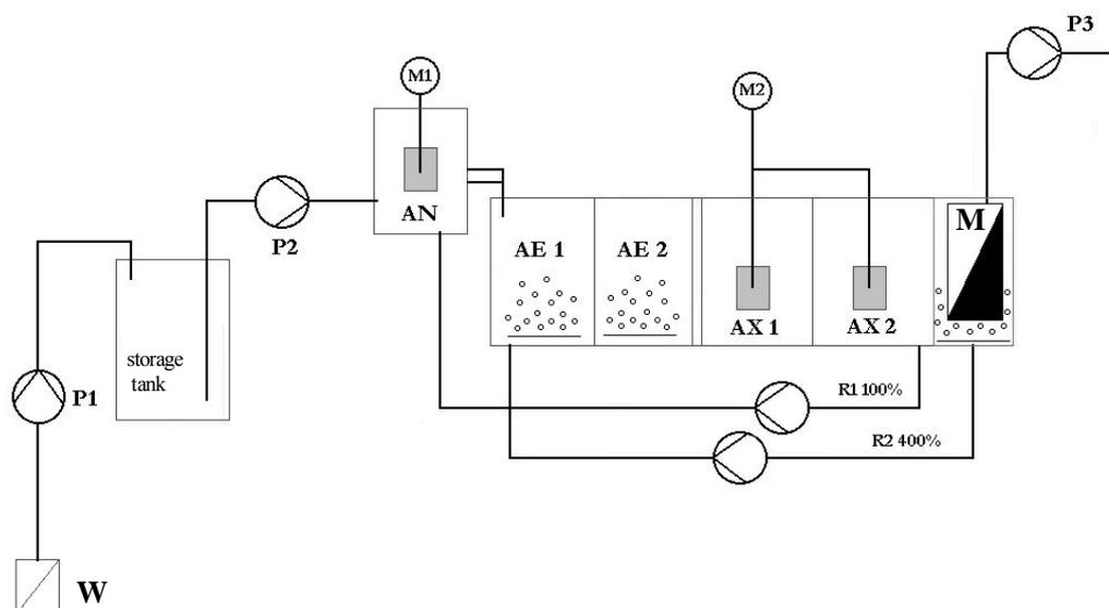
Fig. 1. Plant flow sheet, AN: anaerobic zone, AE: aerobic zone, AX: anoxic zone, M: membrane chamber.
