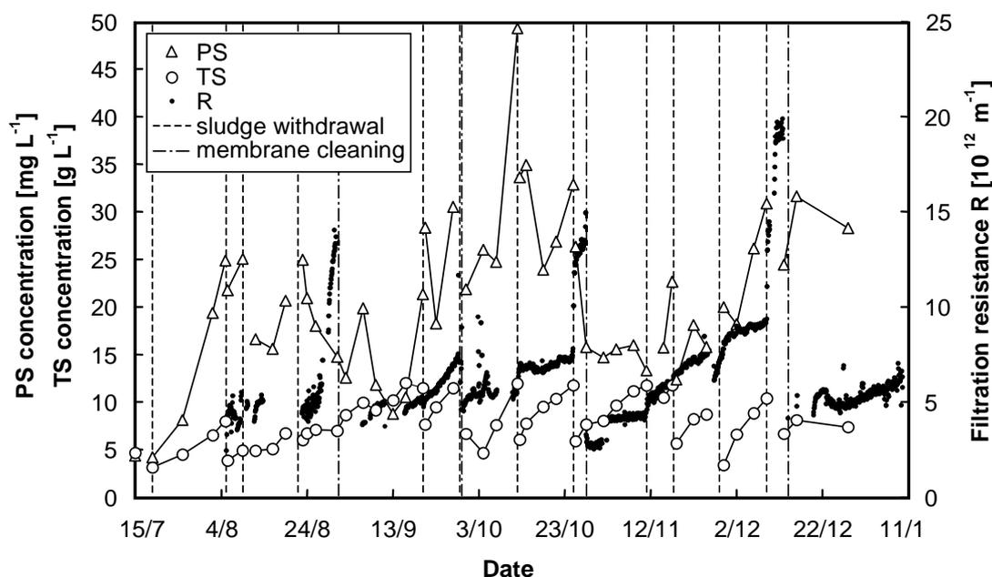
Fig. 2. Development of filtration resistance, biomass (TS) and PS concentration over time.
