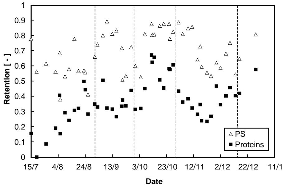
Fig. 5. Retention of PS and proteins over operation time (--- membrane cleanings).
