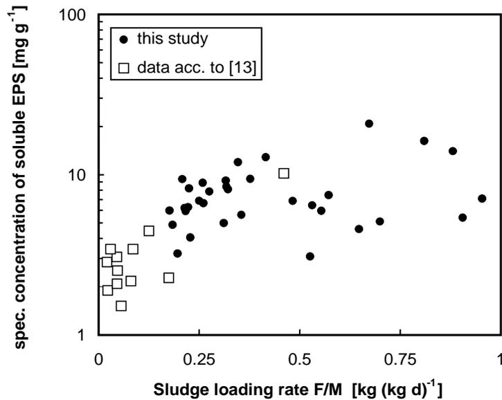
Fig. 6. Specific concentration of soluble EPS as a function of sludge loading rate.
