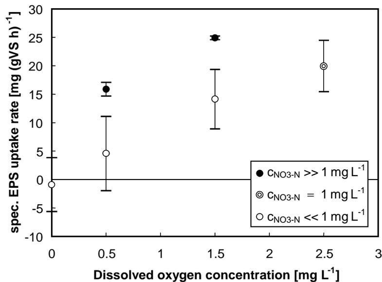
Fig. 4. Specific EPS uptake rate as a function of dissolved oxygen and nitrate concentration (bars represent the measured ranges of uptake rates which result from changing EPS concentration over approx. 24h of operation at each DO concentration).
