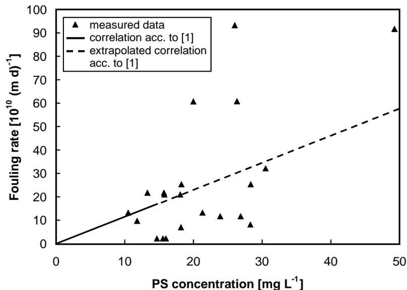
Fig. 7. Fouling rate as a function of polysaccharide concentration.
