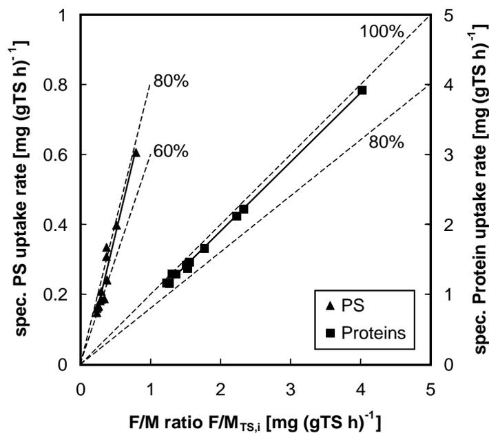
Fig. 8. Specific uptake rates of PS and proteins as a function of respective sludge loading rate.
