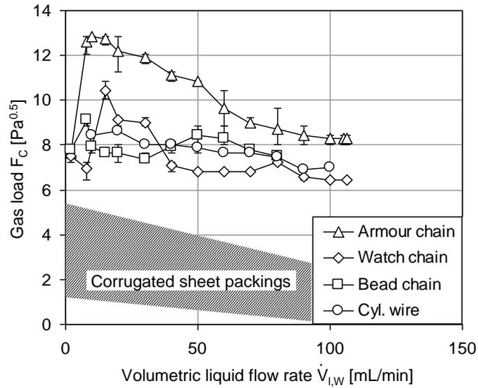
Fig. 4. Load limits at flooding for different single wire geometries.
