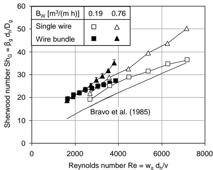
Fig. 8. Dimensionless gas-side mass transfer characteristics for different liquid loads. Comparison of single wire and wire bundle experiments and a correlation for structured packings of Bravo et al. [7].
