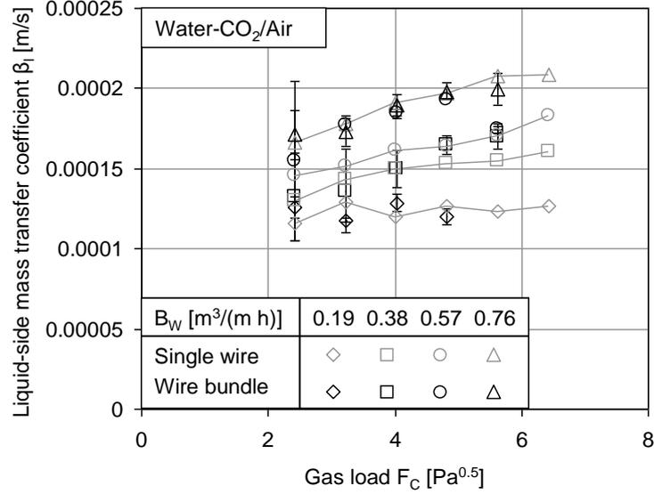
Fig. 9. Liquid-side mass transfer coefficient depending on the gas load for different liquid loads. Comparison of single wire and wire bundle experiments.
