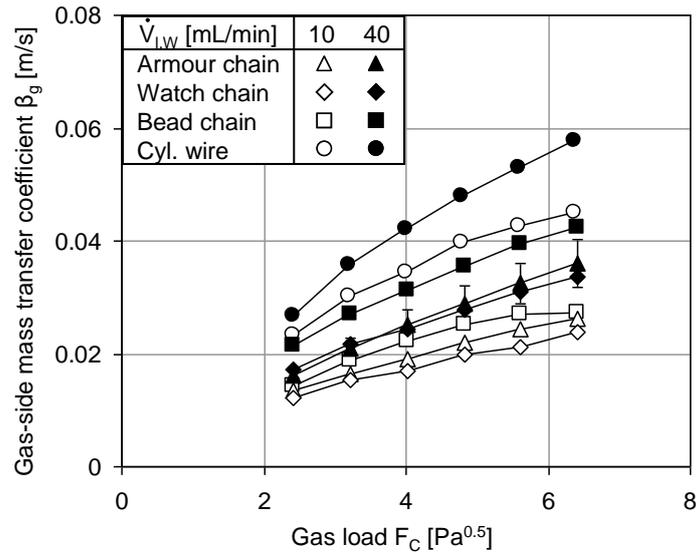
Fig. 7. Gas-side mass transfer coefficient for different wire geometries depending on the gas load for different liquid loads.
