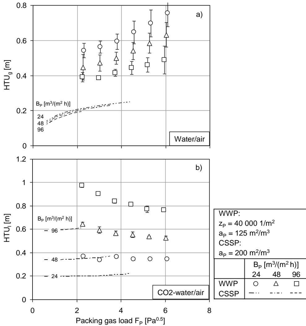
Fig. 10.  $HTU$  value estimation for a) gas-side mass transfer and b) liquid-side mass transfer depending on the packing gas load for different packing liquid loads for a wetted wire packing. Comparison with a correlation for a corrugated sheet structured packing (CSSP) of Rocha et al. [9, 10].
