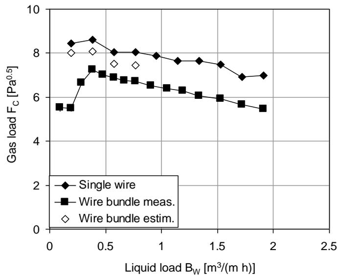
Fig. 5. Load limits for the single wire and the wire bundle. Estimated values for the wire bundle derived from the single wire data considering void fraction and liquid hold-up.
