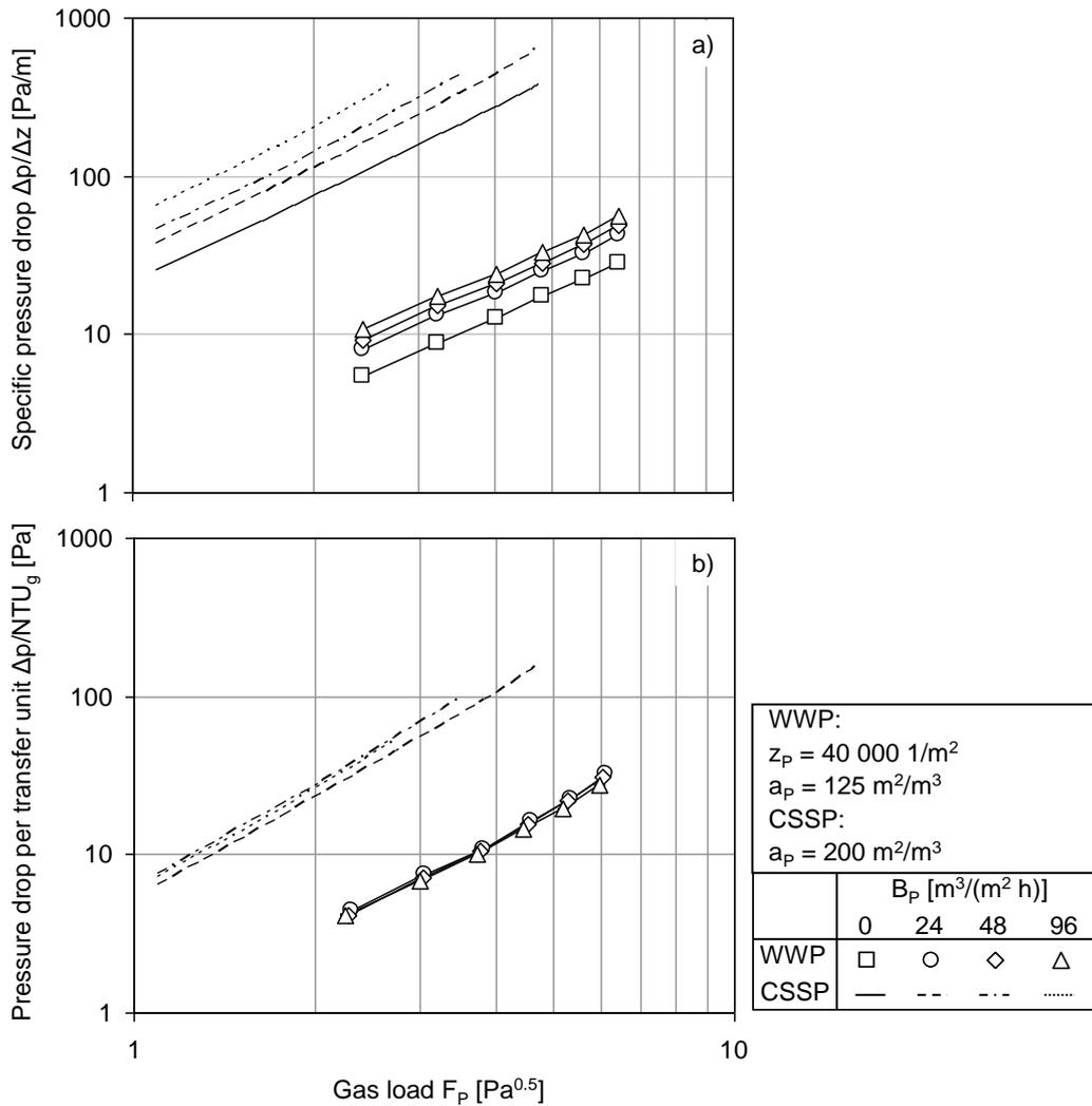
Fig. 11. Estimation of specific pressure drop (a) and pressure drop per transfer unit (b) depending on the gas load for different liquid loads for a wetted wire packing (WWP). Comparison with a correlation for a corrugated sheet structured packing (CSSP) of Rocha et al.[9, 10].
