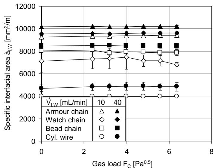
Fig. 6. Specific effective surface area of different wire geometries depending on the gas load for varying liquid loads.
