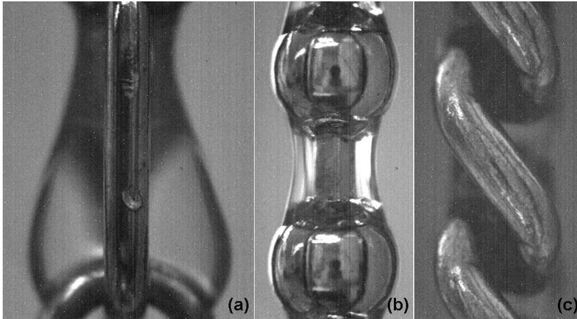
Fig. 3. Liquid film on (a) watch chain (b) bead chain and (c) armour chain.
