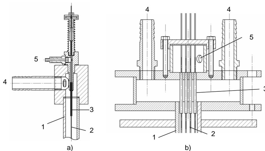
Fig. 2. Construction details of channel head section for a) single wire and b) wire bundle experiments. 1: glass channel, 2: wire (chain), 3: liquid distributor tubing, 4: air exit, 5: liquid inlet.
