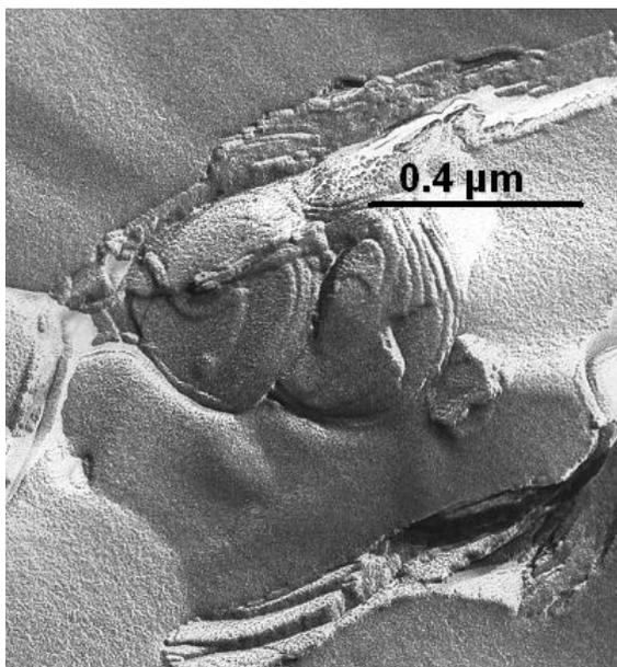
Fig. 8. Electron micrograph of the freeze-fractured NLC dispersion, high-pressure homogenized at 1500 bar for 5 cycles.
