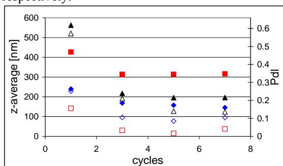
Fig. 3. Mean particle diameter (z-average - full symbols) and Polydispersity index (PdI - open symbols) of formulations homogenized at 500 bar with different residence times.  $\blacktriangle$ : tripalmitin (PPP)  $\blacksquare$ : propylene glycol monostearate (PGMS),  $\blacklozenge$ : middle chain triacylglyceride oil (MCT)
