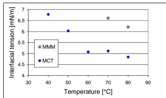
Fig. 2. Temperature dependent interfacial tension between the molten trimyristin (MMM) and the emulsifier solution as well as the triglyceride oil (MCT) oil and the emulsifier solution obtained by pendant drop measurement.
