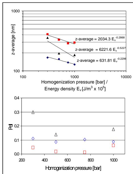
Fig. 4. Mean particle diameter (z-average - full symbols) and polydispersity index (PdI - open symbols) of formulations homogenized for 5 cycles at different pressures.  $\blacktriangle$ : tripalmitin  $\blacksquare$ : propylene glycol monostearate,  $\blacklozenge$ : middle chain triacylglyceride oil
