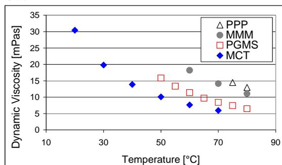
Fig. 1. Temperature dependent dynamic viscosity of the molten lipids and the oil.
