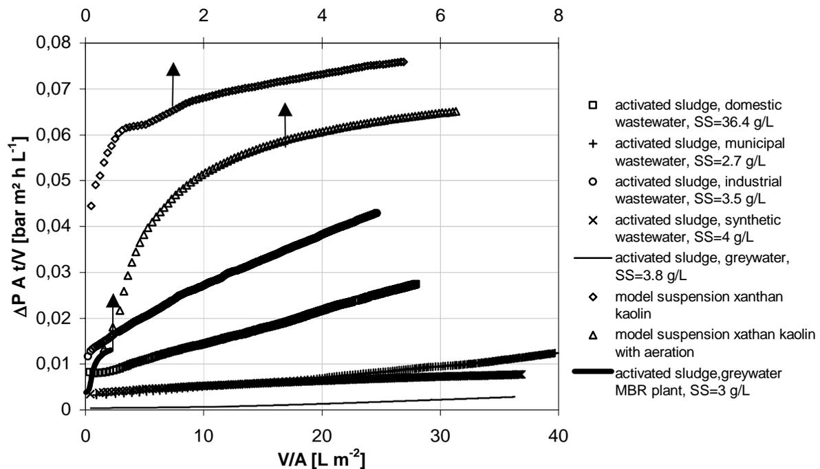
Figure 1: Representation of data according to the dead-end cake filtration model (SS-suspended solids)
